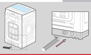
**Note** The opening must not be obstructed by carpeting when the washing machine is installed on a carpeted floor. Drain faults will result if the drain hose is blocked.
