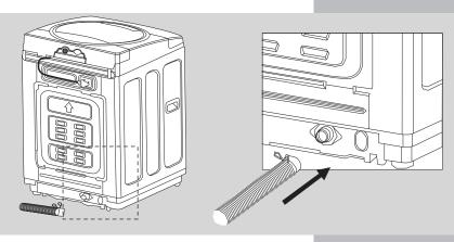
**Note** The opening must not be obstructed by carpeting when the washing machine is installed on a carpeted floor. Drain faults will result if the drain hose is blocked.
