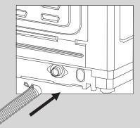
**Note** The opening must not be obstructed by carpeting when the washing machine is installed on a carpeted floor. Drain faults will result if the drain hose is blocked.
